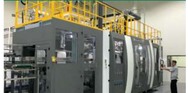
Dual head blow molding machine - Singapore
